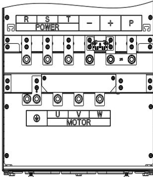
Figure 4-11: 132kW G3 main circuit terminal
