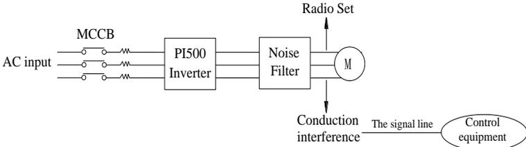
(1) Inductive interference countermeasure : in addition to the installation of noise filter , it can also import the output cables to grounded metal tube. The distance between the output cable and signal line is greater than 30cm , the influence of inductive interference is also significantly reduced . As shown below :
