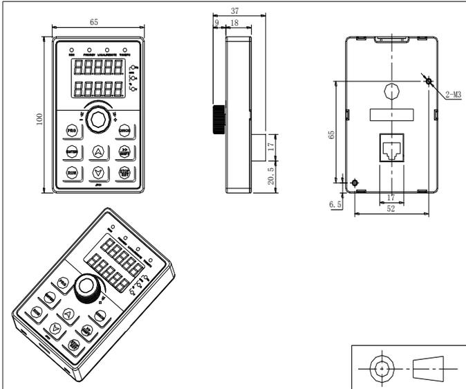
Figure 7-11: PI500 keyboard size (Size: Mm)
