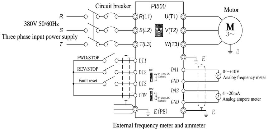
External frequency meter and ammeter
