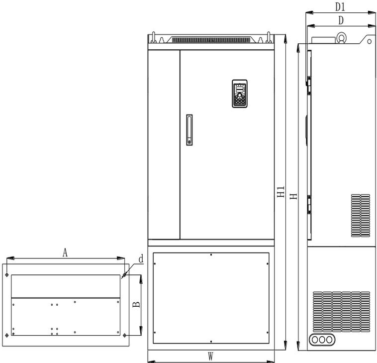
Figure 7-8: 250~400kW G3 (With DC reactor and base)Dimension
