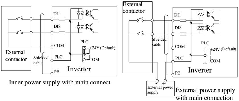
Figure 4-16: Signal input terminal circuit- dry contact mode
