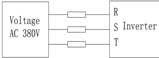
Figure 8-1:380V Drive equipment charging circuit example
