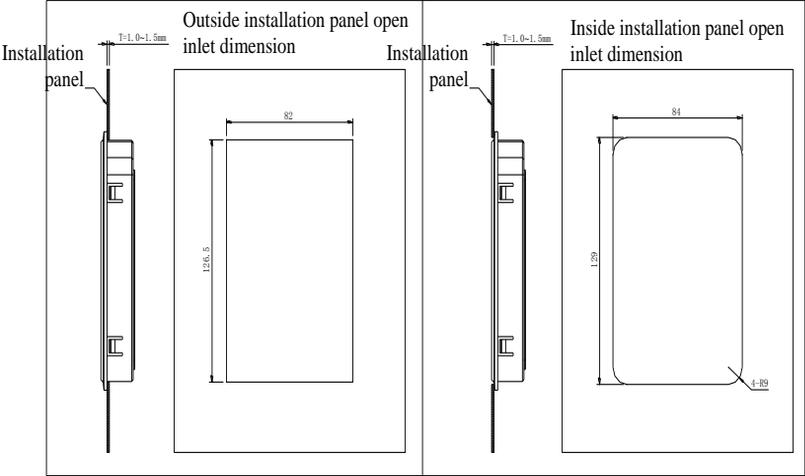
Figure 7-13: Keyboard installation opening size chart (Size: Mm)
