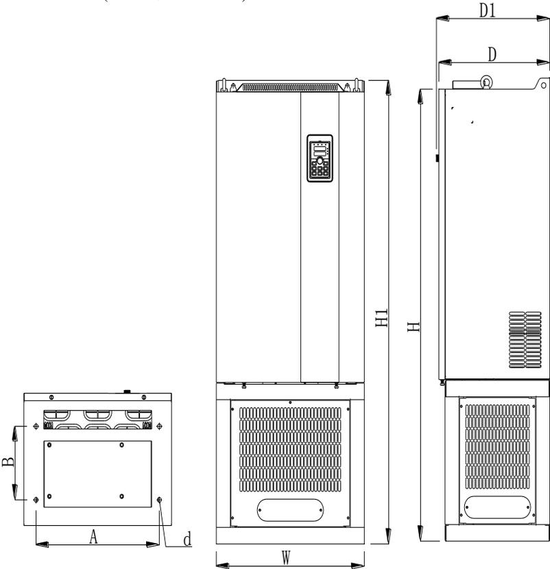
Figure 7-7: 132~220kW G3 (With DC reactor and base)Dimension
