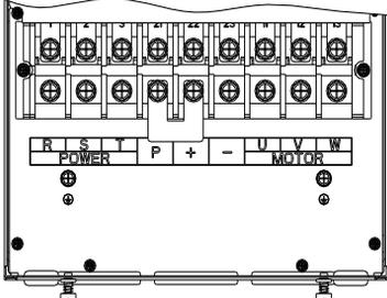
Figure 4-9: 45~75kW G3 main circuit terminal
