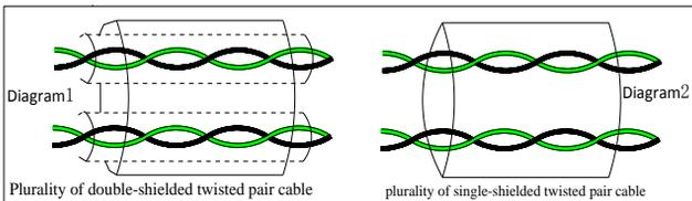
For low-voltage digital signals, double-shielded cable is the best choice, but can also be a single-shielded or unshielded twisted pair, as shown in Figure 2, however, the frequency of the signal, it can only use a shielded cable.
