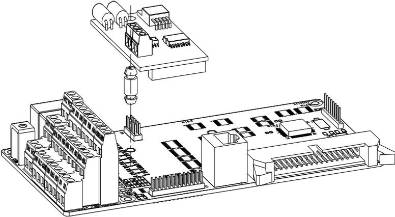
Figure IV-1: CAN bus communication card's installation on SCB
