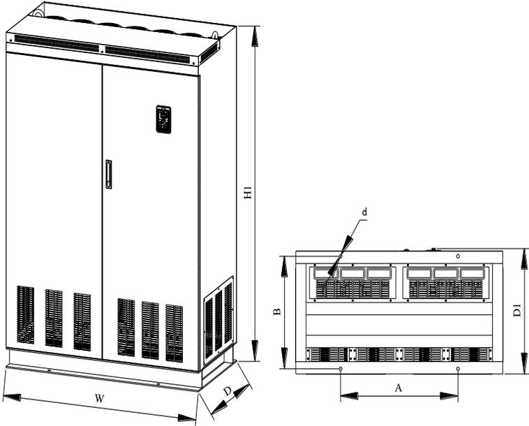
Figure 7-10: 450~630kW G3(DC reactor)Dimension
