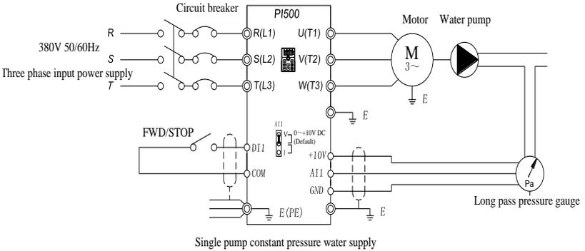
Note: Check the wiring is correct, close the circuit breaker, the inverter power, press the forward button for 1-2 seconds and then stop, check the pump running direction, if the direction is reversed, then change the motor wiring phase sequence
